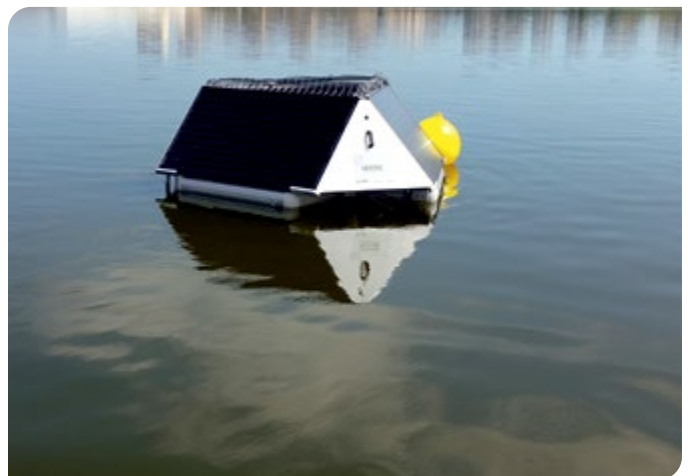
Figure 1: The MPC-Buoy uses ultrasound technology and real-time water quality monitoring to control algal blooms.
