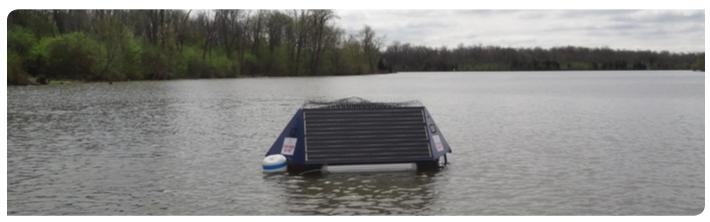
Figure 1: MPC-Buoy algae control system installed in Canoe Brook reservoir #1
