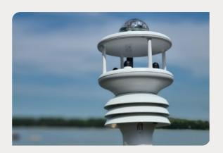
LG Sonic Weather Station is a low maintenance unit that enables more accurate algal bloom predictions by integrating local weather data into the MPC-Buoy and MPC-View software.
