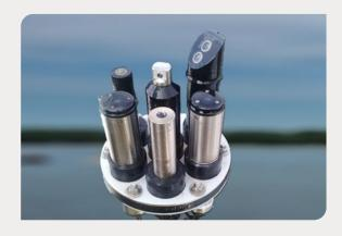
Advanced measurements with smart sensors. The sensors will be protected by an appropriate casing. The sensors are equipped with a wiper mechanism for automatic cleaning after each reading, keeping the maintenance to a minimum.
